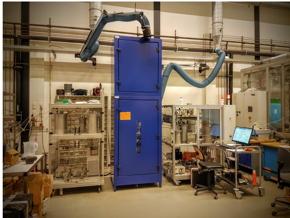
Biphasic Reactor, Continuous, 1-10 L/h
